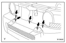
(b) Using a clip remover, remove the 5 clips.
