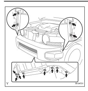
(c) Remove the 8 screws and the 4 bolts.
